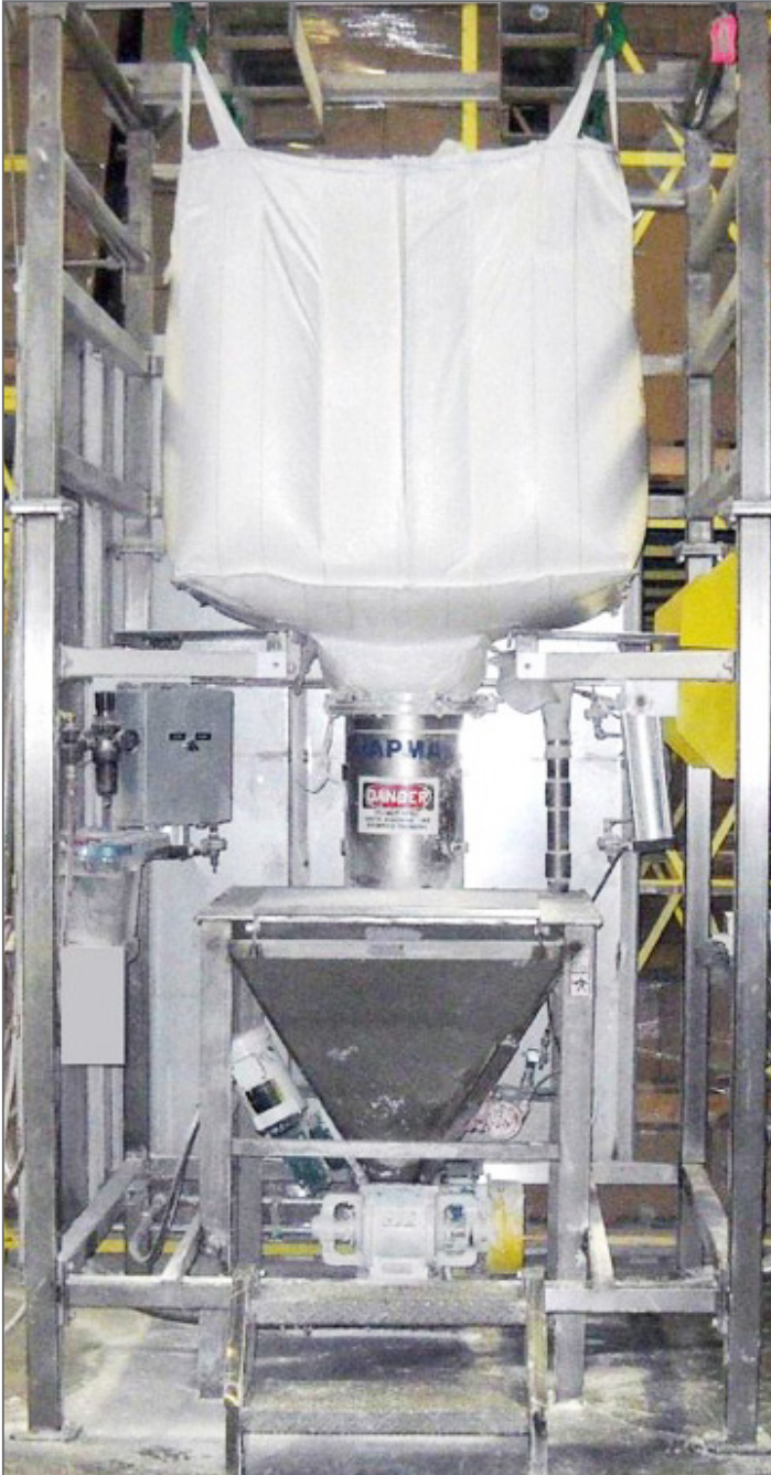
Basic American Foods underwent a major reconfiguration of its Blackfoot, Idaho operations to increase capacity within a very short time frame. One process affected by the project included a previously purchased Hapman bulk bag unloader (top) to supply corn starch to two, new pneumatic vacuum conveyors.
