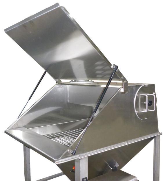
The SR Series Dust Collector can be integrated with an existing hopper for point-of-process dust containment. Reverse-pulse-jet automatically cleans the filter and puts all ingredients back in the process.
