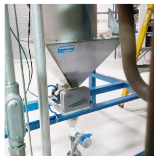
The patent pending HBRP wastewater treatment system at the Village of Gilbert's facility used a Hapman Bulk Bag Unloader with integral feeder as the ballast delivery system.
