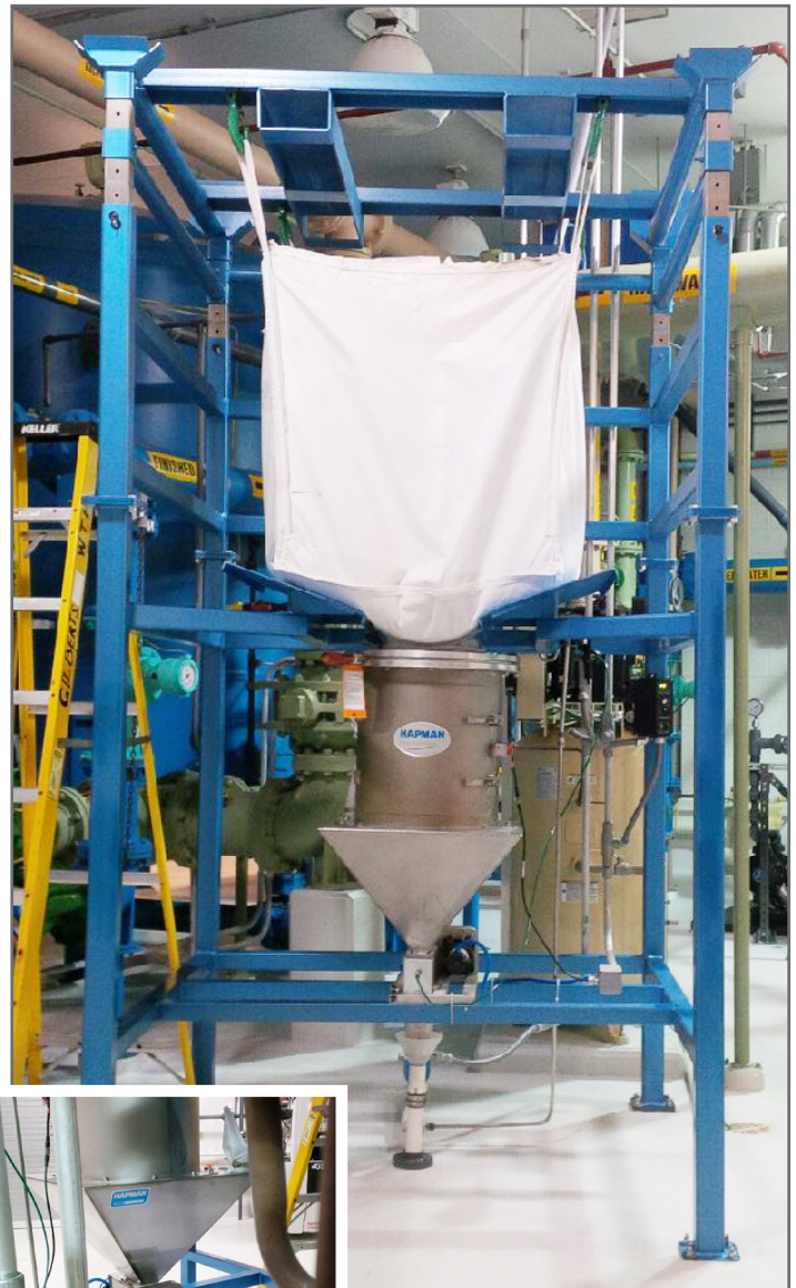
The patent pending HBRP wastewater treatment system at the Village of Gilbert's facility used a Hapman Bulk Bag Unloader with integral feeder as the ballast delivery system.
