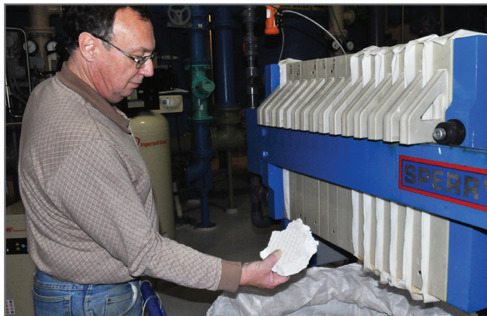
The solid Barium/Radium captured from the wastewater treatment process designed by Baxter & Woodman.
