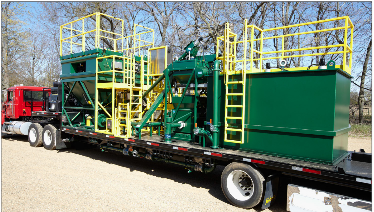
Hapman's mobile mixing system provided a capability that many other companies can not do - the ability to mix dry chemicals at the job site as needed.
