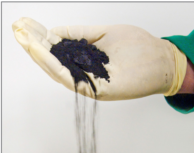
Carbon dust impregnated with platinum and palladium material is smelted in the furnace leaving behind the precious metals.
