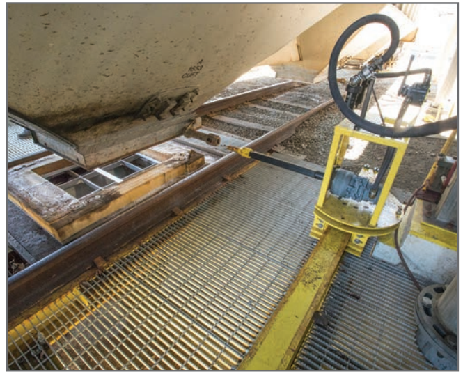
Railcar interface seals the discharge of the railcar.
