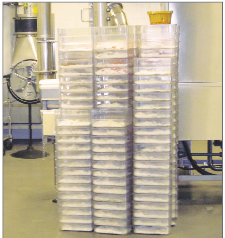
The GlaxoSmithKline facility cleans approximately 3,500 small animal cages per week. The high volume and sticky nature of the waste animal bedding was difficult to move pneumatically; clogging the conveyor frequently.
