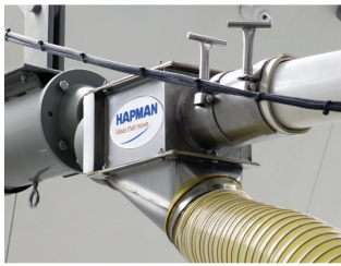
Pictured above is the Helix conveyor motor suspended from a trolley mounted to the ceiling at the Guixens Food Group plant in Tampa Florida.
