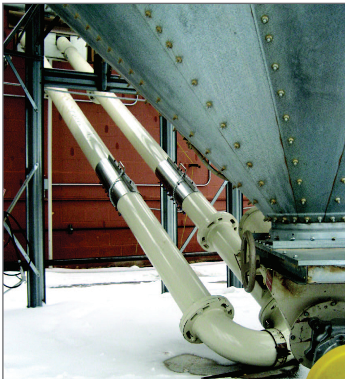
Hapman's tubular drag conveyor reliably and gently moves 52,000 tons (47,174 metric tons) of pelletized fuel from the exterior storage silo to the interior packing line annually.
