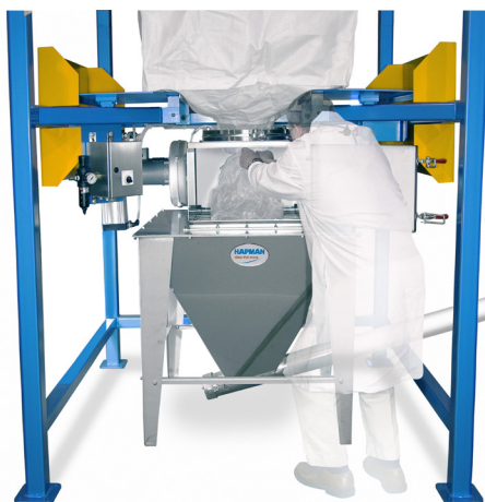
Iris Valve & Tie Box allows for easy access and tight shut-off at bag spout when new or empty.
