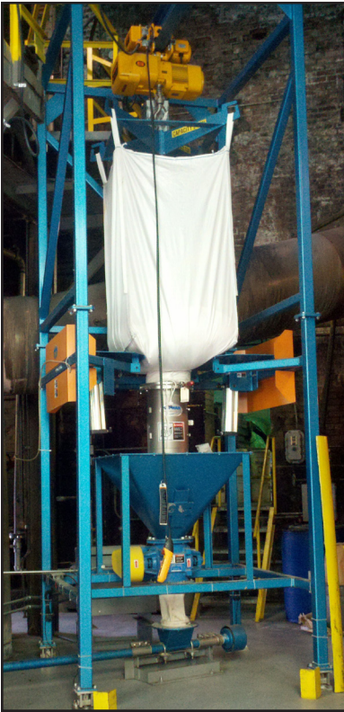
Hapman's Loss-in-Weight Bulk Bag Unloader optimized batching operations and alleviated the physical strain of manually handling bulk bags, which eliminated health, housekeeping, and product loss issues associated with material dusting.
