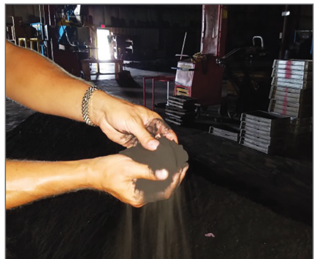
Manually shoveling sand to fill cope and drag boxes is physically demanding for mold makers.
