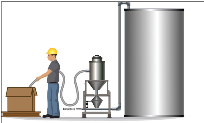
Slurry with a vacuum conveyor to direct slurry.
