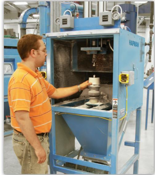
*Knock out station with specially designed apparatus and integral dust hood reduces dust created during the plaster knock-out process, preventing equipment problems and improving the work environment.*
