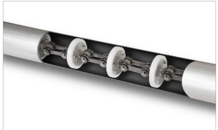
Hapman's Sealed-Pin type, are precision-machined and assembled by compressing elastomeric washers into the hinge point of the chain, which minimizes the opportunity for material presence there (very important when handling certain materials).
