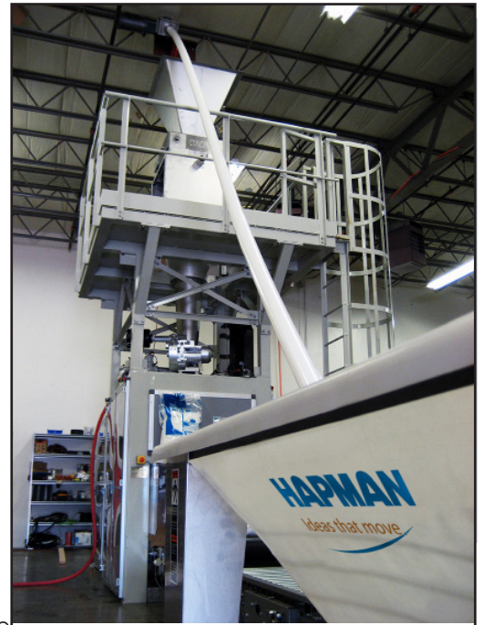
Hapman's 300 Series Helix flexible screw conveyor with polyurethane hopper and flat wire auger conveys plastic pellets 28 feet (8.5 meters) to the TB 1200 form-fill-seal solution.
