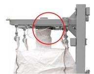
Venturi Bag Inflation Inflates the bag to maximize capacity by removing folds and creases in the bag prior to filling.
