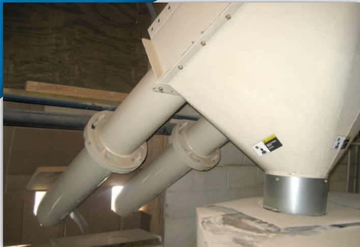
The 40 ft (12.2 m) tubular drag discharges pellets into the packaging hopper. Accumulated dust from the former rubber belt conveyor sits on top of the packaging hopper.
