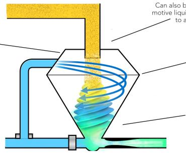
Can also be used to add a liquid to a motive liquid stream, or to add powder to a motive gas stream.
