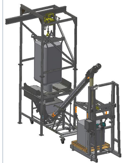
3D engineering file from Hapman engineers depicting bulk bag unloader emptying into the Helix® before refilling a smaller bulk bag.
